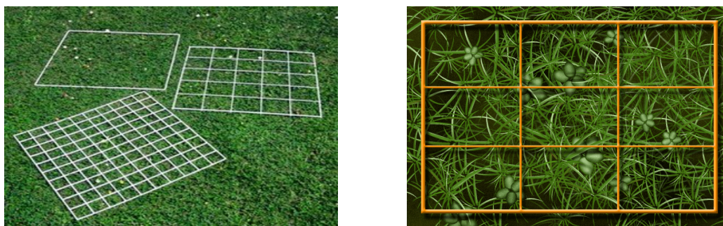
Figure 1. Frame quadrat (left) and Photograph frame quadrat (right) method for estimation of vegetation cover.
